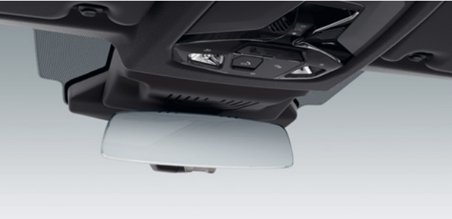
□ Interior and exterior mirror package, including automatic dimming interior and driver's side exterior mirrors and electric fold-in function for exterior mirrors.
