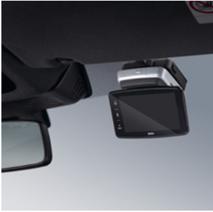
o The QHD and full HD cameras of the BMW Advanced Car Eye 3.0 Pro automatically record what is happening in front of and behind the vehicle when an incident takes place.
