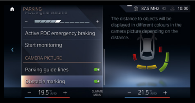
□ The Parking Assistant Plus 2 assistance system has more cameras in addition to the Parking Assistant and also displays the vehicle surroundings in three dimensions. This makes it even easier to monitor the manoeuvre.
