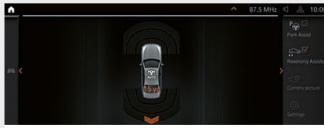
□ The Reversing Assistant\* stores the last 50 m of the driven path in forward travel up to 35 km/h, so that it can be retracted if required. You are relieved of the steering work and can concentrate on monitoring the vehicle environment.
