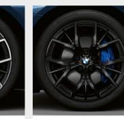
□ 19" M light alloy wheels Y-spoke style 845 M Jet Black with mixed tyres, wheel size front 8J x 19 with 245/40 R19 tyres, wheel size rear 9J x 19 with 275/35 R19 tyres.<sup>2</sup>
