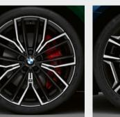
□ 20" M light alloy wheels Y-spoke style 846 M Bicolour Jet Black with mixed tyres and run-flat tyres, gloss-lathed, wheel size front 8J x 20 with 245/35 R20 tyres, wheel size rear 9J  $\times$  20 with 275/30 R20 tvres.4
