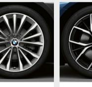
□ 19" light alloy wheels □ 19" M light alloy wheels Y-spoke style 845 M Bicolour W-spoke style 663 Ferric Grey gloss-lathed with mixed tyres Jet Black with mixed tyres, and run-flat properties, front 8J gloss-lathed, wheel size front x 19 with 245/40 R19 tyres, rear 8J x 19 with 245/40 R19 tyres, 9J x 19 with 275/35 R19 tyres. wheel size rear 9J x 19 with 275/35 R19 tyres.<sup>2</sup>
