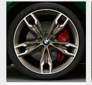
□ 20" M light alloy wheels Double-spoke style 668 M Cerium Grey matt with mixed tyres and runflat tyres, glosslathed, wheel size front 8J x 20 with 245/35 R20 tyres, wheel size rear 9J  $\times$  20 with 275/30 R20 tyres.
