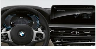
BMW Live Cockpit Professional\* includes two high-quality displays consisting of a 12.3" Control Display and a fully digital 12.3" instrument display.
