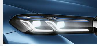
□ In laser high-beam mode, BMW Laserlight\* illuminates a range of up to 650 m, nearly twice as far as that of conventional headlights. Better visibility in the dark significantly increases safety. Blue accents and the lettering "BMW Laser" in the headlight also underline the technological standards and the sportiness of the vehicle.
